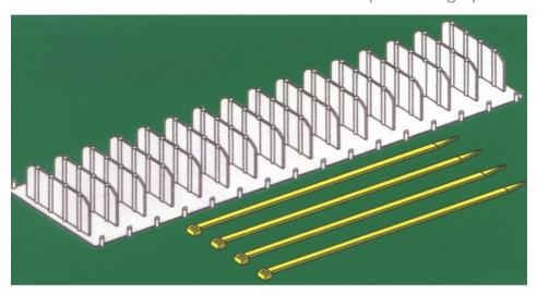
2. Place the OM-S casing spacer module around the pipe so that its outside wall is completely covered. Cut the module strip with a joint gap of approximately 5 mm so that it does not overlap.
